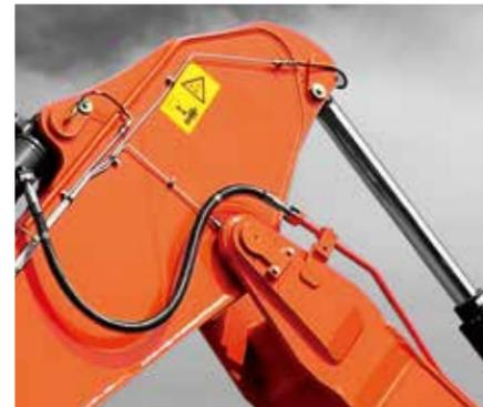
The adaptability to harsh dust work conditions has been improved by increasing the lubrication point of the arm connection unit.
